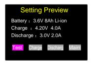
If the parameters are correct, users can select the four listed in the menu according to their task requirement functions. Use <Up>, <Down> and <Enter> to select and run.
