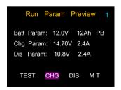
If the parameters are correct, users can select the four listed in the menu according to their task requirement functions. Use <Up>, <Down> and <Enter> to select and run.
