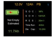
When you charge battery from nonempty state, after full charged, it can get an estimated capacity
