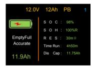
When you charge battery from empty state, after full charged, you will get an accurate capacity.
