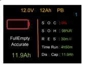
When discharge battery from full charged state, after discharged empty, it will get an accurate capacity.
