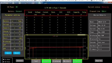
For example, to charge a single 3.7V lithium battery, click "Single charge":
