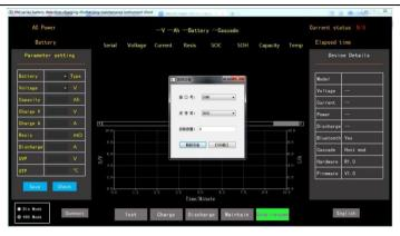
If the item bar of "Serial Port Number"(串口号) is blank, please click the lower left corner to "refresh the device"(刷新设备), or the inverted triangle identifier on the right side of the item bar will pop up the corresponding serial port number. Note: The serial port number is slightly different according to the computer model. Set "Baud Rate"(波特率) to 9600. "Cascading Quantity"(级联数量) Set this parameter based on site requirements.
