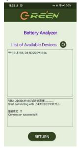
Note: Once the BM device is successfully connected to the mobile phone or tablet computer through Bluetooth, the function keys on the BM panel will be temporarily frozen and disabled. At this time, only the function keys in the mobile phone or tablet APP can control the battery settings and function operation of the BM. When the APP program is terminated and closed, the BM panel keys can resume their normal functions.
