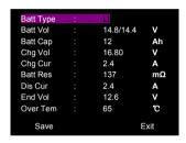
At this time, press the "Down" key twice, the "LI" on the right side of the battery type becomes "PB", and the corresponding voltage and other parameters will also change accordingly, as shown in the following figure.
