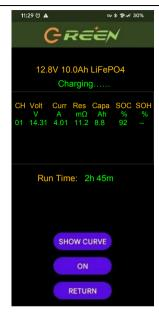
After charging or discharging done, click the [SHOW CURVE] button to enter the charging and discharging curve viewing interface. Click [SHOW CURVE] button again, return the earlier main data view screen.
